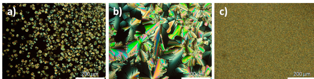
Figure 2. Microphotographs of the textures observed by POM for (a) T3C 4 -TPC 10 , Col h , 85 °C (cooling), (b) T3C 4 -TPC 6 , Col h , 117 °C (cooling), and (c) T3C 4 -TPC 4 , Col h , room temperature (after annealing above the glass transition).
